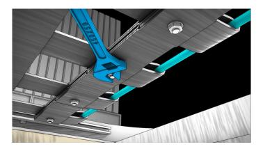
Remove detent pen and slide cover between the 1" and 2" drilled holes and re-insert the detent pin from the bottom and secure. Latch each lanyard to the closest t- Bolt. Repeat on the other side.
